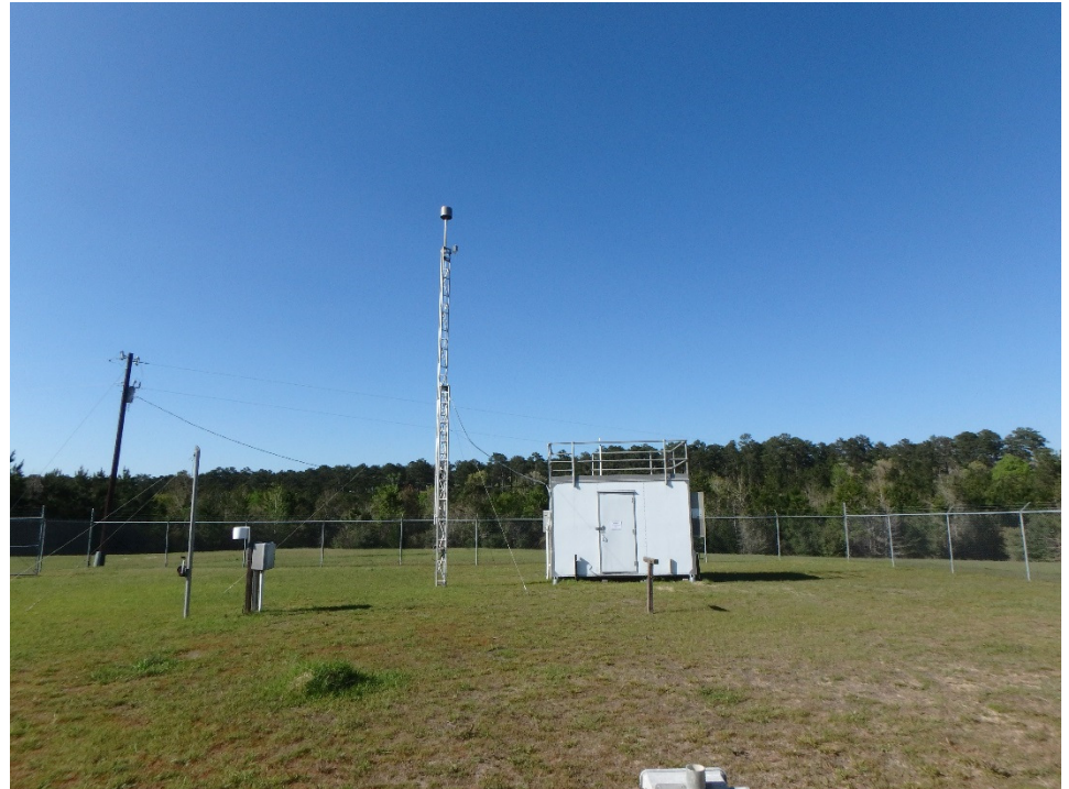
Alabama-Coushatta, TX CASTNET site (ALC188). Filter pack, O 3 and temperature is collected by EPA.
